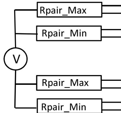
FIG. 33-#<sub>7</sub> Unbalanced source configuration
