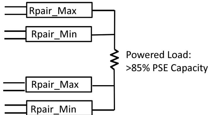
FIG. 33-#<sub>3</sub> Unbalanced load configuration
